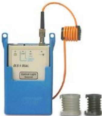
Figure 1: Reference Cable Wrapped Around a Mode Filtering Mandrel (Courtesy; Noyes Fiber Optics)
