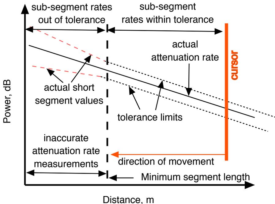
Figure 4: Details of Minimum Length Determination
