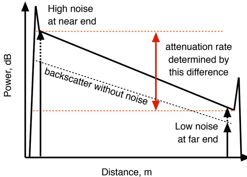
Figure 3: Attenuation rate With High-Low Noise at Opposite Ends of Fiber
