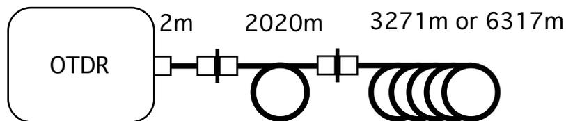
Figure 2: Test Set Up
