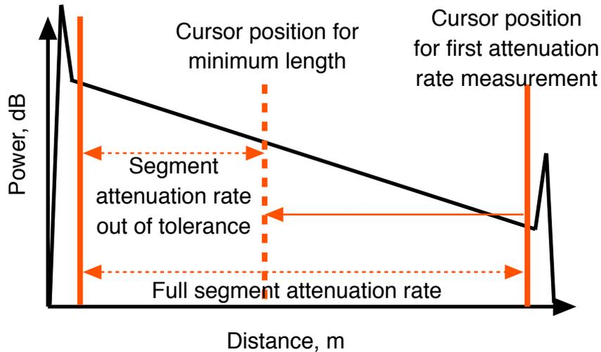
Figure 3: Cursor Positions for Full and Minimum Length Attenuation Rates
