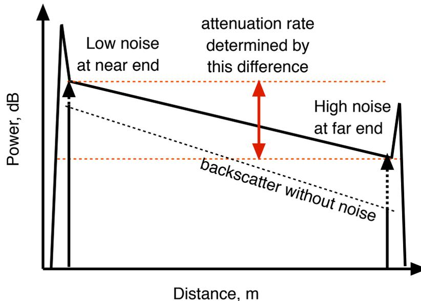
Figure 4: Attenuation rate With Low-High Noise at Opposite Ends of Fiber
