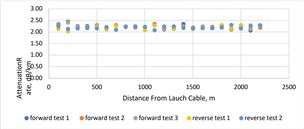
Figure 2: 100m Sub-Segment Attenuation Rate Vs. Distance from OTDR Launch Cable
