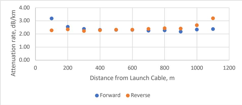
Figure 1: 100m Sub-Segment Attenuation Rates Vs. Distance from Launch Cable
