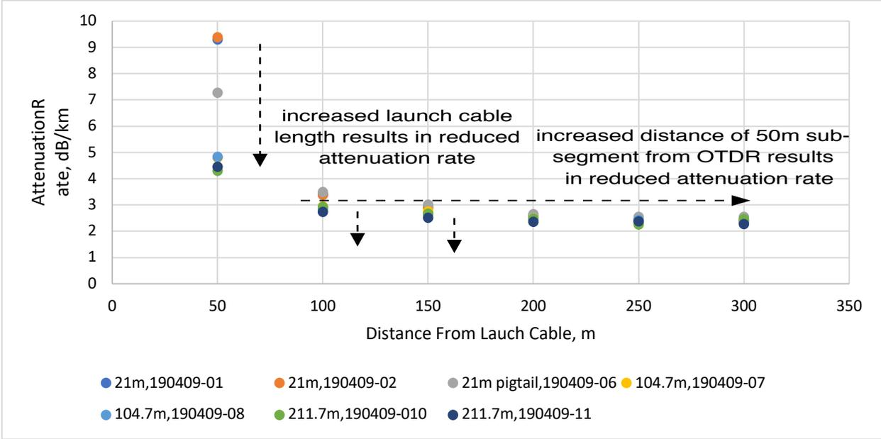
Figure 3: Attenuation Rate of ~50m Subsegments Vs. Distance from OTDR With Different Length Launch Cables
